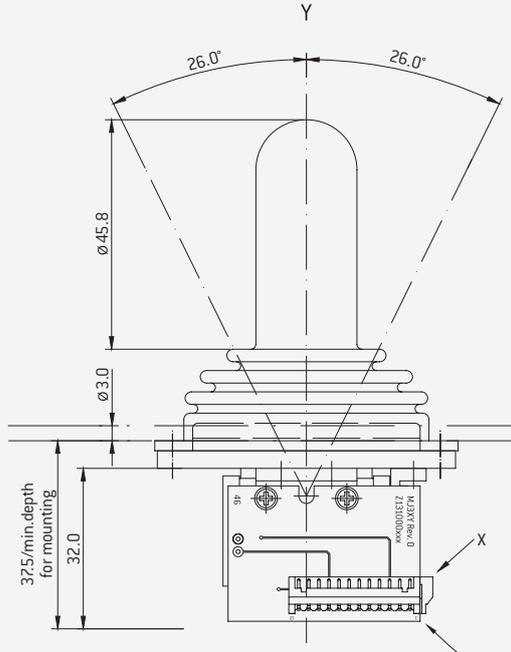
Assembly into Housing from Inside / Screw Head outside of housing
